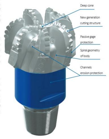
Sometimes bits are equipped with additional row of diamond cutting structure for maximum covering and severalfold increase of operating life. During creation of bits for hard rocks are used diamond cutters of increased impact and abrasion resistance that are selected according to accumulated information on tool performance in the region of operations.
