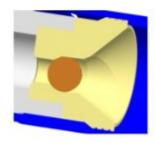
Bit activation is carried out by means of easy drillable ball. Upon reaching TD dropped ball plugs hole and under pressure the drillable center moves forward and blades expand.
